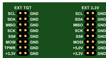
Figure 6: The External Connectors provides the developer with a quick and easy way to interface or monitor any or all of the Level Shifter Board signals on either the Adapter/Analyzer side or the target side.
