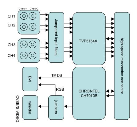
The device is controlled using i2c from the fpga.
