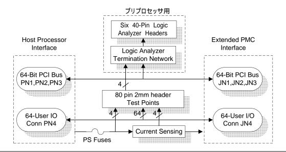
The extender/analysis probe permits extension of a PMC card beyond the edge of a host processor front panel, providing access to both Side 1 and Side 2 of a PMC under test. Support is provided for the 64-bit PCI bus and connection for the 64 rear user I/O signals, as well as operation up to 66 MHz clock.
