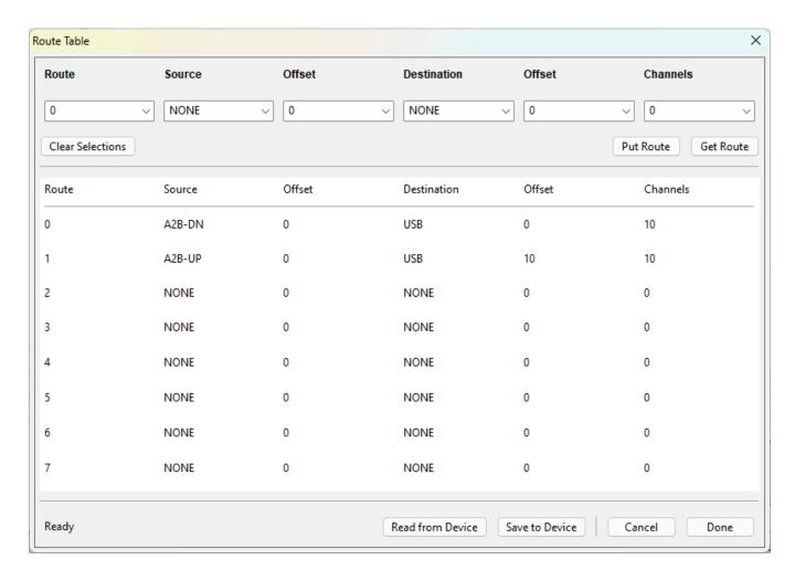
To configure additional routes, select the Route number, Source + Offset, Destination + Offset, and Channels in the upper section of the dialog box and press the **Put Route** button.
