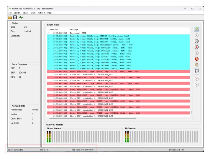
At this point, the A<sup>2</sup>B Bus Monitor is ready to start monitoring A<sup>2</sup>B bus activity as shown above.
