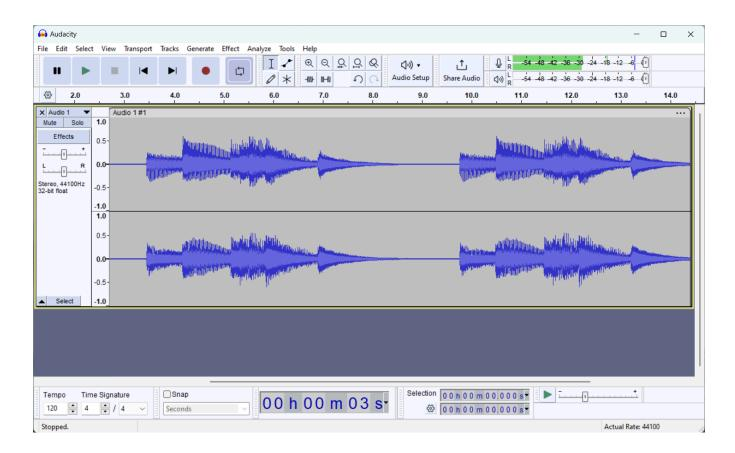
Example of Audacity recording the two A2B-DN channels that were routed to USB in the previous section, <u>Audio Routing in the Bus Monitor GUI.</u> In the Audio Setup, select the Microphone (Flextech AKT Bus Monitor) as the recording device.
