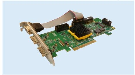
The Gidel HawkEye-CL frame grabbing and real-time image processing system provides the core infrastructure required to support the most demanding Vision and Imaging applications.
