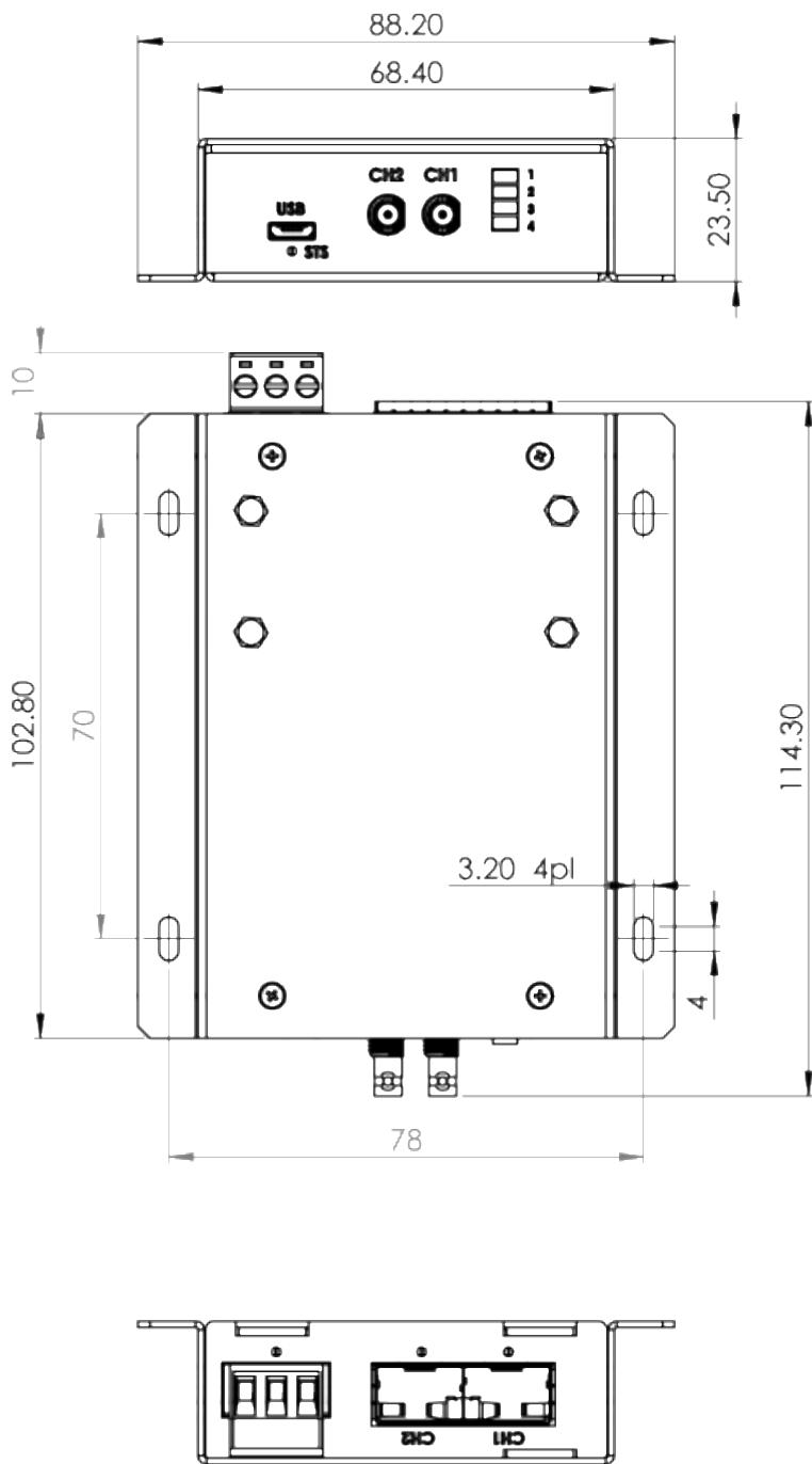
Dimensions are in millimeters.
