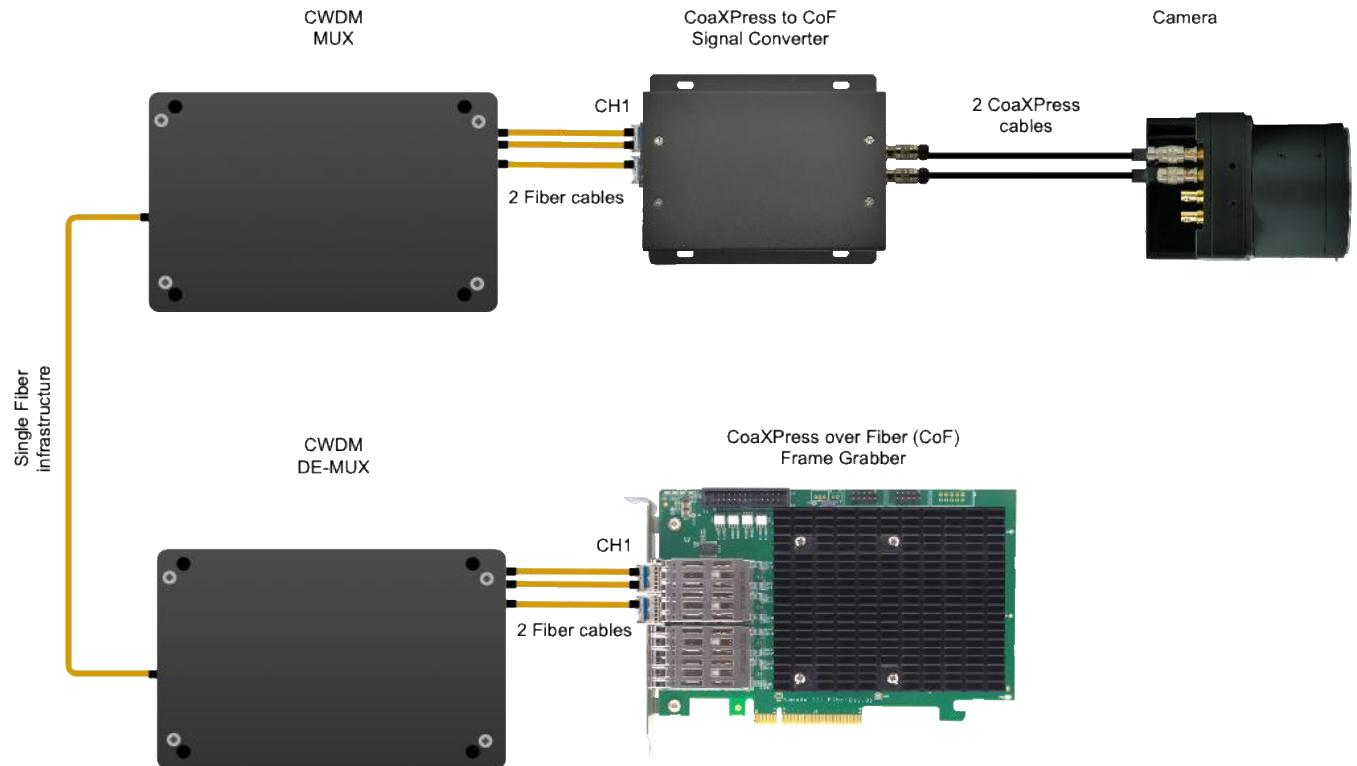
**NOTE:** Channel 1 (CH1) must have a duplex fiber connection (Or BIDI SFP with single fiber cable) while other channels can have a simplex fiber connection from device side to host.
