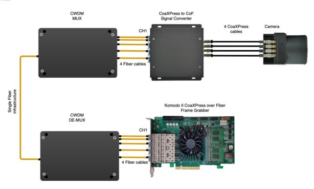
**NOTE:** Channel 1 (CH1) must have a duplex fiber connection (Or BIDI SFP with single fiber cable) while other channels can have a simplex fiber connection from device side to host.
