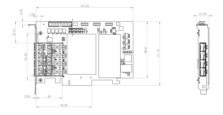
Dimensions are in millimeters.
