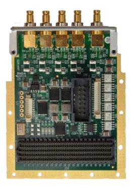
Up to 5 host/device links can be provided using front panel DIN 1.0/2.3 connectors. Each link supports standard CoaXPress bitrates up to 6.25 Gbps. Each host link is capable of providing up to 13W of power to compatible devices via Power over CoaXPress (PoCXP). The FMC-CXP can support up to 5 individual links, or combinations of aggregated CoaXPress links (e.g. one camera requiring one link, and two additional cameras each using two links).
