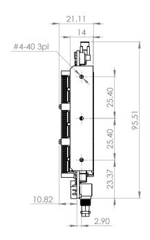
Dimensions are in millimeters.
