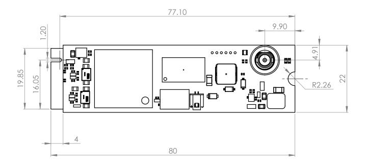
Dimensions are in millimeters.
