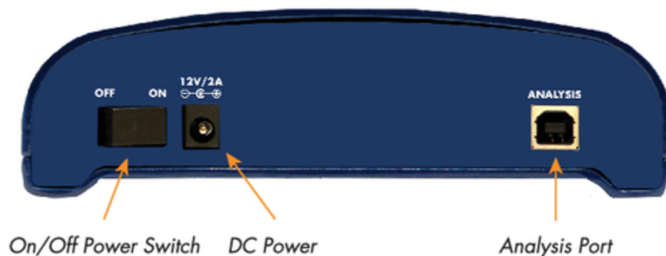
Figure 2 : Beagle USB 5000 Protocol Analyzer – Back Panel
