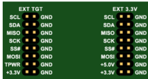
Figure 7 : The External Connectors provide the developer with a quick and easy way to interface or monitor any or all of the Level Shifter Board signals on either the Adapter/ Analyzer side or the target side.
