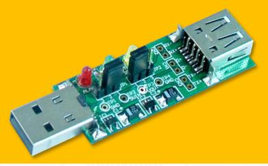
The USB Fixture is a test tool for USB 3.0 interface with multi-functions of voltage swtich, voltage test and current test. It's especially designed to save valuable labor and time in the production environment.
